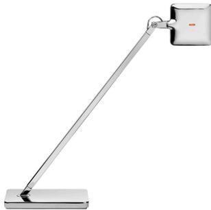
Table lamp providing direct light. Head in pressofused aluminium, diffuser in photo-engraved methacrylate with aluminate surround. Power pack on plug, base in pressofused zamak. Directionable head. ON/OFF switch with Soft Touch technology and light flow adjustment to 2 intensities (100% – 50% – 0%). Power pack on plug with interchangeable plugs.
