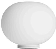
Table/desk lamp providing diffused light. Diffuser consisting of an externally acidetched, hand blown, flashed opaline glass and a die-cast aluminum threaded ring nut with alodine plating finish. 30% fiberglass reinforced injection-molded polyamide base. Gray painted, die-cast aluminum diffuser support. On the cable there is the electronic dimmer which allows the regulation of light brightness.
